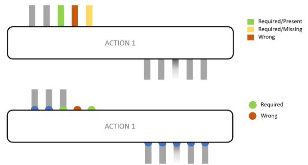
Figure 2: An action-space visualization example, with preconditions at the top of each action, and effects at the bottom. Deletion effects are represented as a flow fading out. Top: The highlight-based explanation visualization; Bottom: The port-based explanation visualization.
